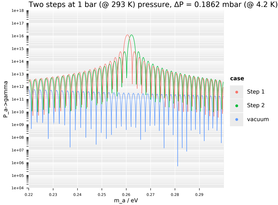
Figure 17: Plot of the vacuum conversion probability depending on the axion mass for the vacuum case and two pressure steps with ^4\text{He} buffer gas at 1 bar at T = 4.2 K.
