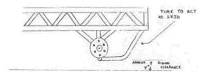
Front axle support to be made of 2.00" x.095" chrome molly tubing or 2.00"
