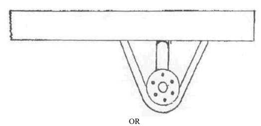
Front axle support to be made of 2.00" x .095" chrome moly tubing or 2.00" x .120" mild steel tubing or same material as tractor frame rails. Front axle support should connect to each frame rail inline and extend toward front of tractor. Front skid/front axle support should have radius to prevent digging into track. Front axle support frame should be strong enough to support front end weight of tractor. Support should have a maximum of 4" ground clearance.
