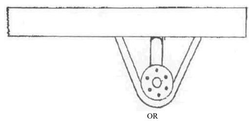
Front axle support to be made of 2.00" x .095" chrome moly tubing or 2.00" x .120" mild steel tubing or same material as tractor frame rails. Front axle support should connect to each frame rail inline and extend toward front of tractor. Front skid/front axle support should have radius to prevent digging into track. Front axle support frame should be strong enough to support front end weight of tractor. Support should have a maximum of 4" ground clearance.
