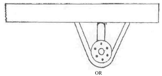
Front axle support to be made of 2.00" x .095" chrome moly tubing or 2.00" x .120" mild steel tubing or same material as tractor frame rails. Front axle support should connect to each frame rail inline and
