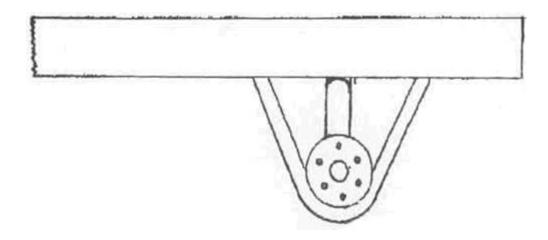
Front axle support to be made of 2.00" x .095" chrome moly tubing or 2.00" x .120" mild steel tubing or same material as tractor frame rails. Front axle support should connect to each frame rail inline and extend toward front of tractor. Front skid/front axle support should have radius to prevent digging into track. Front axle support frame should be strong enough to support front end weight of tractor. Support should have a maximum of 4" ground clearance.
