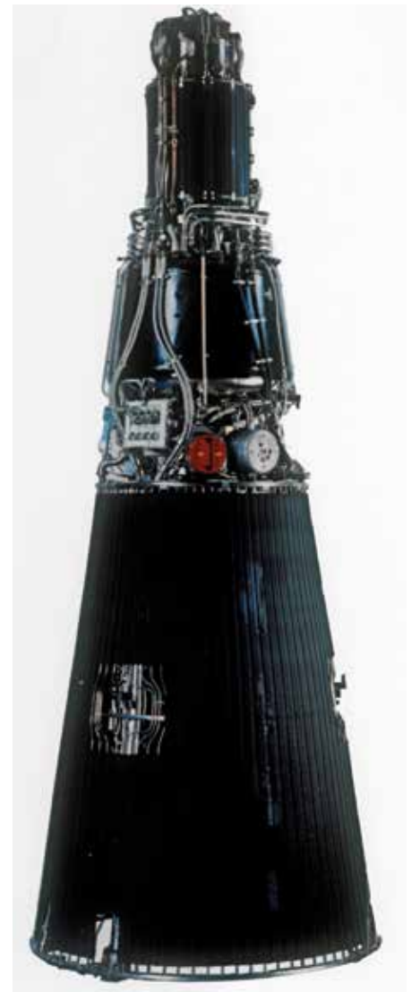
TOPAZ-II reactor system. (Photo: Scott Wold)
