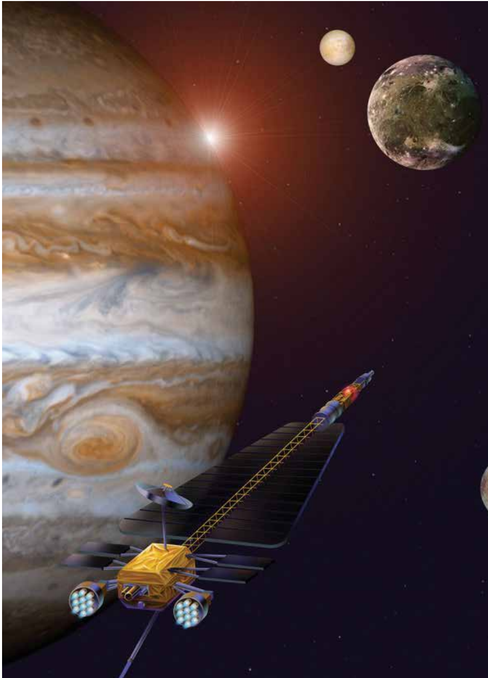
Early concept of Jupiter Icy Moons Orbiter spacecraft exploring Jupiter and its moons. The nuclear reactor and Brayton cycle power plant are located at the front of the spacecraft. The large structure in the middle is the heat rejection system. Two ion thrusters, located at the rear of the spacecraft off of the science platform, provide propulsion. (Image: NASA)
