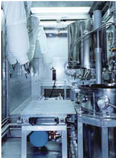
RTG assembly chamber for the GPHS at Mound. (Photo: DOE Flickr)
