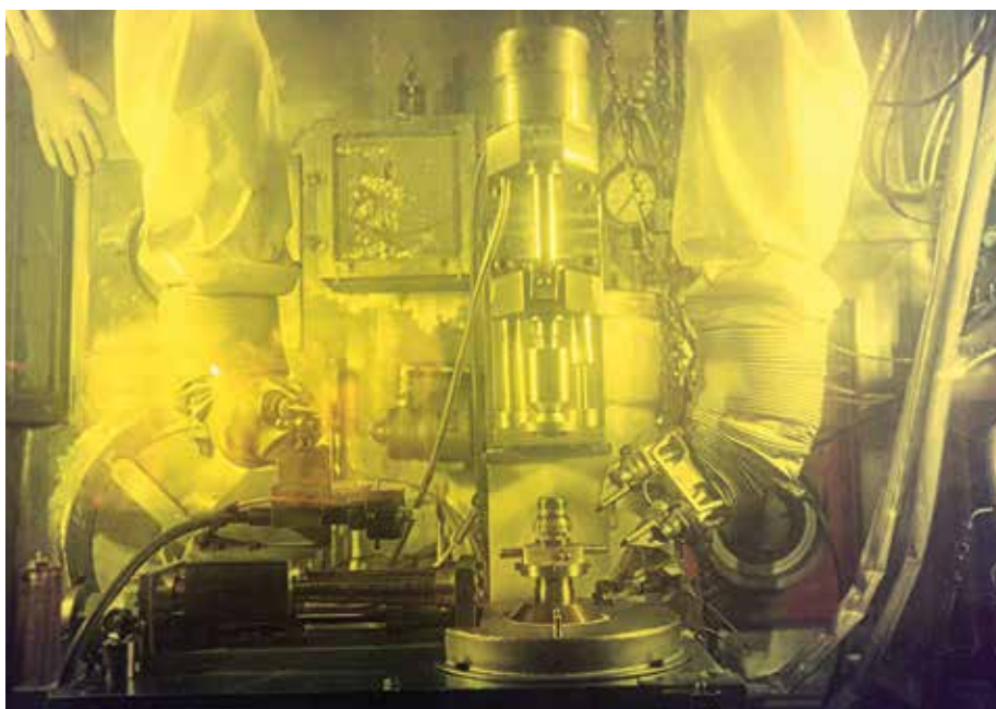
View of hot cell 6 inside the PuFF facility (looking through water-filled shield window), where iridium shell welding operations were performed to encapsulate GPHS fuel pellets. (Photo: SRS Flickr)
